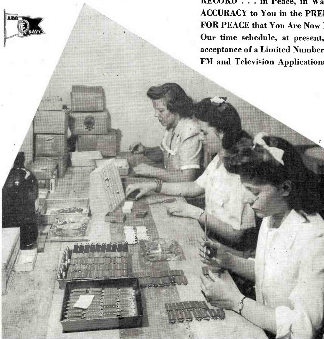
ASSEMBLY ACCURACY —Last Assembly Operation of IF Filter Crystals Before Baking Process Preceding Final Electrical and Sealing Tests.
